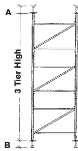
3 Tier High Aluma Frame® with standard Item #514 Screwjack top and bottom.
